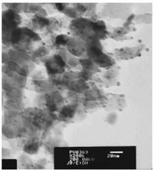
The real gold content in the nanocomposites prepared, determined by AAA is 0.8, 2.5 and 9 wt %. The specific surface area values of the samples are similar and vary between 40 and 46  $m^2/g$ . The TEM observation shows а homogeneous incorporation of gold nanoparticles in the ZnO matrix and narrow nanoparticle size distribution. The average diameter of Au-NPs in the samples, estimated from TEMmicrographs is  $4 \pm 0.3$  nm.
